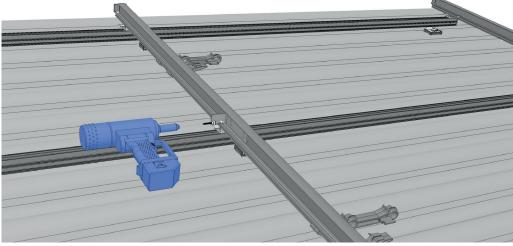
Rivet the Alu angle bracket into the pre-drilled holes. Use the two supplied pop rivets for mounting. The rivets are mounted using the rivet pliers. It is important to use a rivet nosepiece for the IMS-Solar
