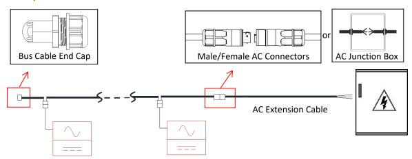
When AC extension cable is needed, users could connect the AC bus cable and AC extension cable in a junction box or use a pair of male/female AC connectors that APsystems provides as optional accessory.
